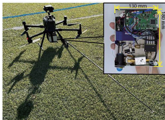
Fig. 2 Drone mounting a ball SAW GC with a 3 m long sampling unit
