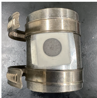
Fig.4 Optical image of flexible sensor fixed with curved surface using hose clamp
