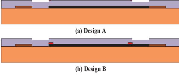
Fig. 4 Ditches in TC-SAW structures.
