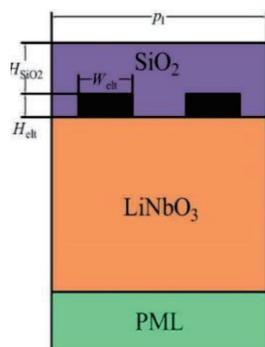
Fig. 1 Cross-section of resonator structure
