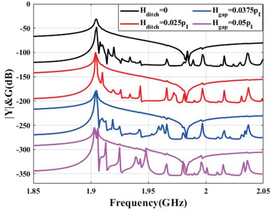
Fig. 5 Variation of  $G$  and  $Y$  of Design A with  $H_{\text{ditch}}$ .
