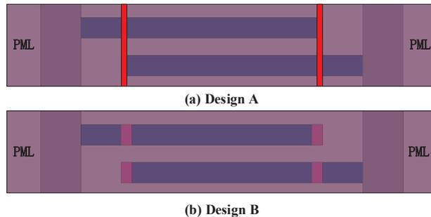
Fig. 2 Top view of two piston mode designs colored in red: (a) Design A: Cu stripes, and (b) Design B: Cu dots.
