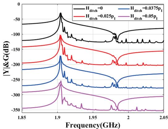
Fig. 6 Variation of  $G$  and  $Y$  of Design B with  $H_{\text{ditch}}$ .
