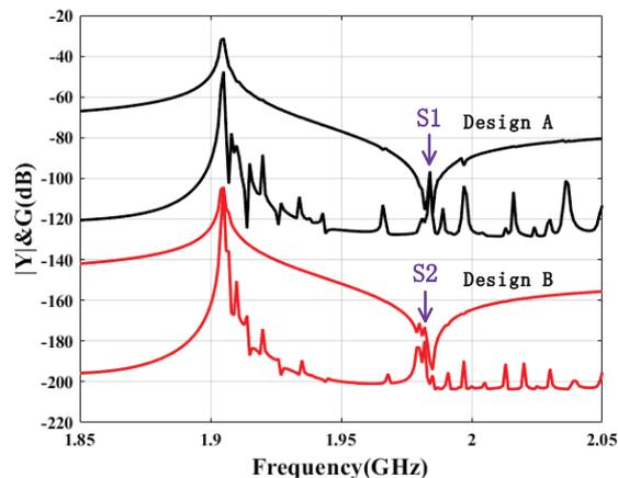
Fig. 3 Calculated admittance and conductance of designed resonators
