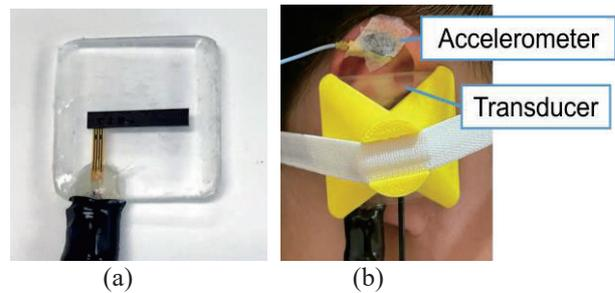
Fig. 1 (a) A homemade transducer. (b) Presentation position of accelerometer and transducer.
