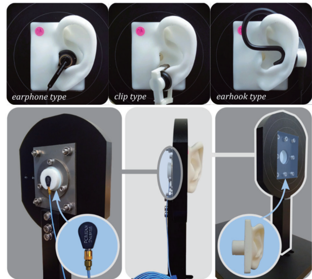
Fig. 1 Top panel: Vibrator in three different pinna locations. Bottom panel: Mounting base with accelerometer placement behind the ear canal.
