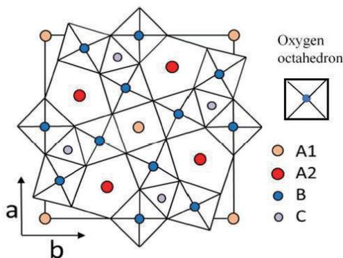
Fig. 1 Crystal structure of tetragonal tungsten bronze ferroelectrics on the (001) plane.
