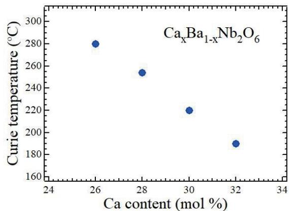
Fig. 2 Ferroelectric Curie temperatures of calcium barium niobate crystals.
