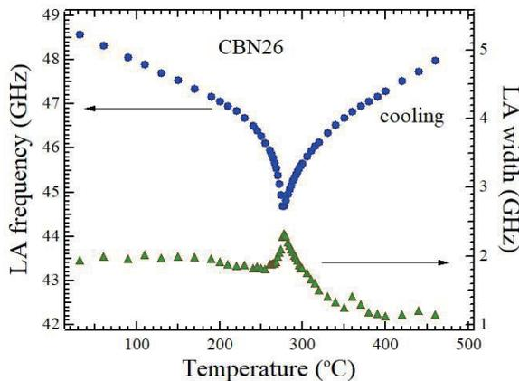
Fig. 3 Temperature dependence of LA frequency shift and width on cooling along the ferroelectric  $c$ -axis of a CBN26 crystal.
