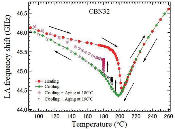
Fig. 4 Temperature dependence of LA frequency shift which propagates along the ferroelectric  $c$ -axis of a CBN32 crystal. Aging is observed at 180 and 190°C.
