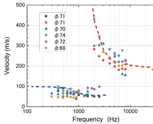
Fig.4. Measured velocity as a function of frequency for six samples of Japanese radish with diameters of 68,70, 71, 71, 72 and 74 mm. Blue and red dashed lines indicate the fitted curves of the fundamental and second modes, respectively.
