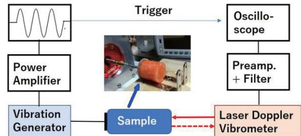
Fig. 1 Experimental system for measuring the velocity of acoustic pulsed waves propagating in fruits and vegetables. The inset shows a cylindrical watermelon sample attached to an oscillator.
