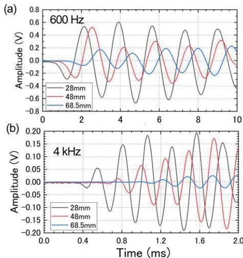
Fig. 2. Pulsed waves detected for three different lengths of watermelon at 600 Hz (a) and 4 kHz (b).
