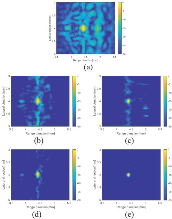
Fig. 2. B-mode images by; (a) simple averaging; SCM with (b) no-compression and (c) compression; CF compounding with (d) no-compression and (e) compression.
