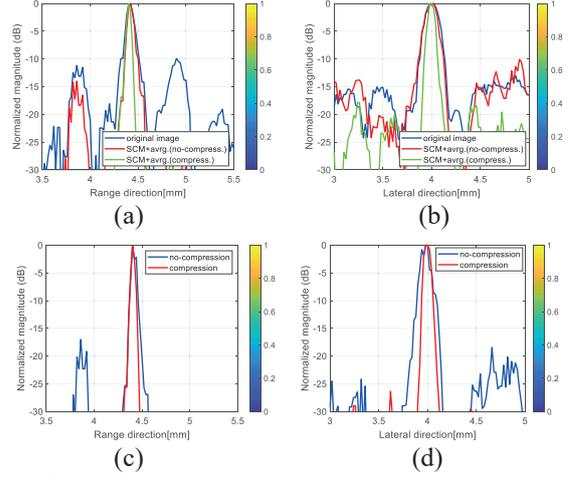
Fig. 3. Amplitude profile with simple averaging in (a) range direction and (b) lateral direction; with CF compounding in (c) range direction and (d) lateral direction.
