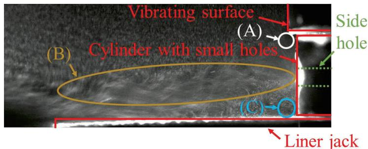
Fig. 5 Particle behavior around cylinder with small holes (5,000 fps).
