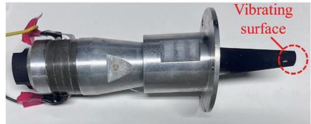
Fig. 2 Vibration source (Freq.: 28 kHz).
