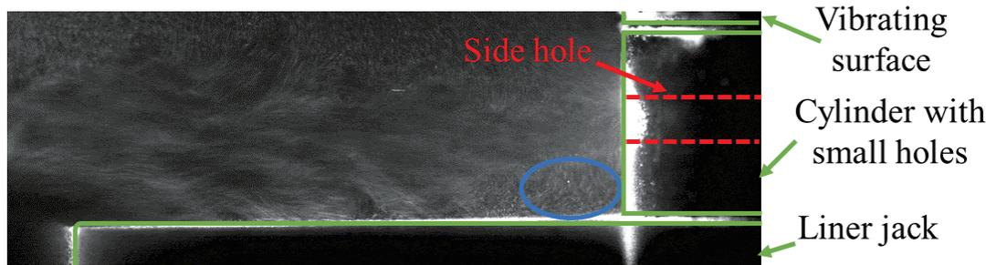
Fig. 7 Particle behavior around cylinder when not levitated (5,000 fps).
