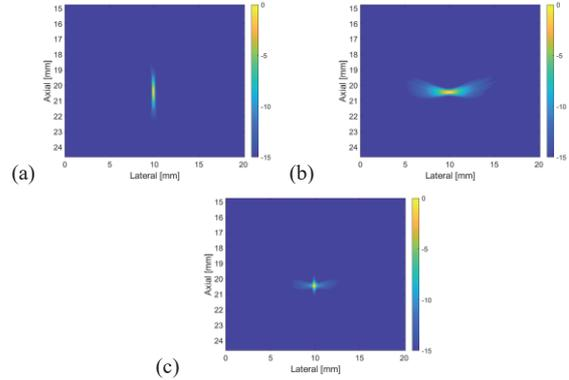
Fig. 2 B-mode images: (a) Time-reversal imaging with multiple signal classification (TR-MUSIC); (b) DAS using profiles of R-MUSIC; (c) Combination of R-MUSIC and TR-MUSIC (Proposed method).
