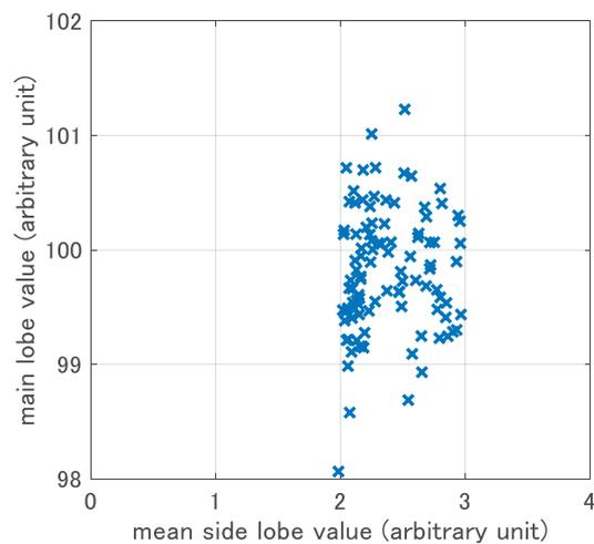
Fig. 2 Main lobe peak value and side lobe mean value of generated pulse trains.
