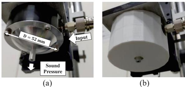
Fig. 1 Picture of (a) uncovered and (b) covered T-DPLUS.
