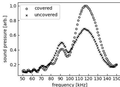
Fig. 6 Frequency characteristics of covered and uncovered T-DPLUS.
