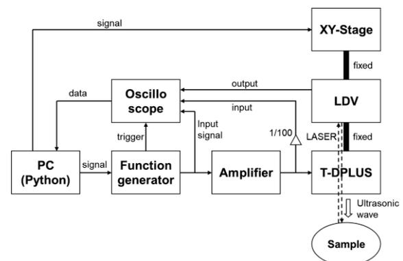
Fig. 3 Firmness measurement system.
