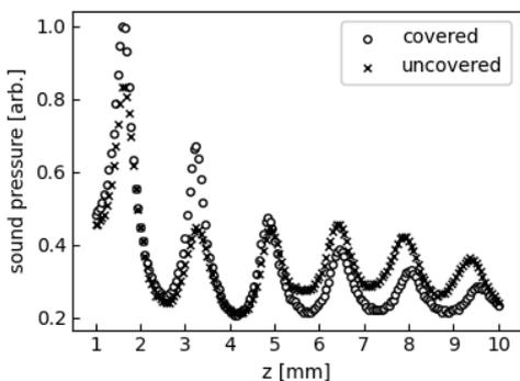
Fig. 5 Distance characteristics of covered and uncovered T-DPLUS.
