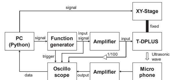
Fig. 2 Measurement system of acoustic pressure characteristics of T-DPLUS.
