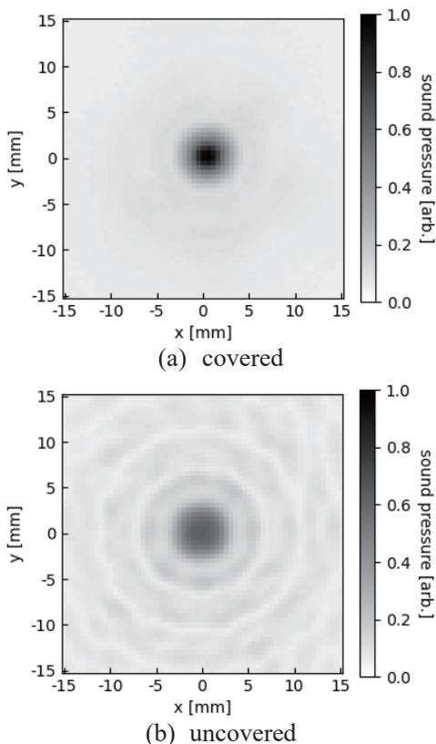
Fig. 4 Sound pressure distribution of covered and uncovered T-DPLUS.
