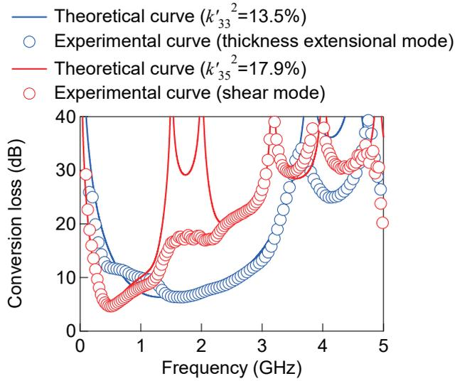
Fig. 4 Conversion loss curves of PbTiO<sub>3</sub>-HBAR
