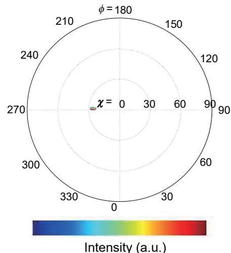
Fig. 2 (002) XRD pole figure of c-axis tilted epitaxial PbTiO<sub>3</sub> films of SrTiO<sub>3</sub> 25° off-angle substrates
