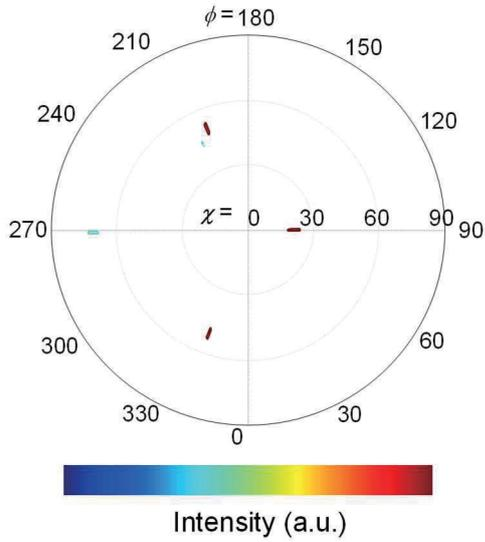
Fig. 3 (101) XRD pole figure of c-axis tilted epitaxial PbTiO<sub>3</sub> films of SrTiO<sub>3</sub> 25° off-angle substrates
