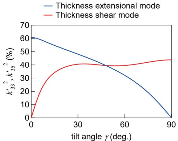
Fig. 1 Relationship between c-axis tilt angle and electromechanical coupling coefficient  $k'_{33}{}^2$  and  $k'_{35}{}^2$  of PbTiO<sub>3</sub>
