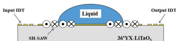
Fig. 1 Schematic illustration of the SH-SAW propagation at a liquid/solid interface
