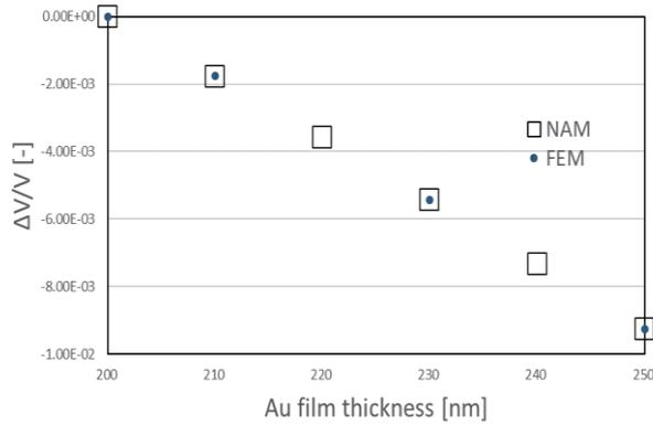
Fig. 2 Velocity change as a function of gold thickness
