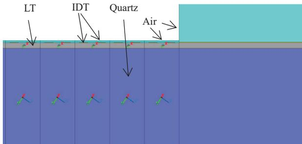
Fig. 4 Cross section of the IDT and the propagation path
