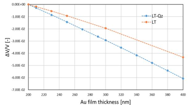
Fig. 5 Velocity change in bonded structure
