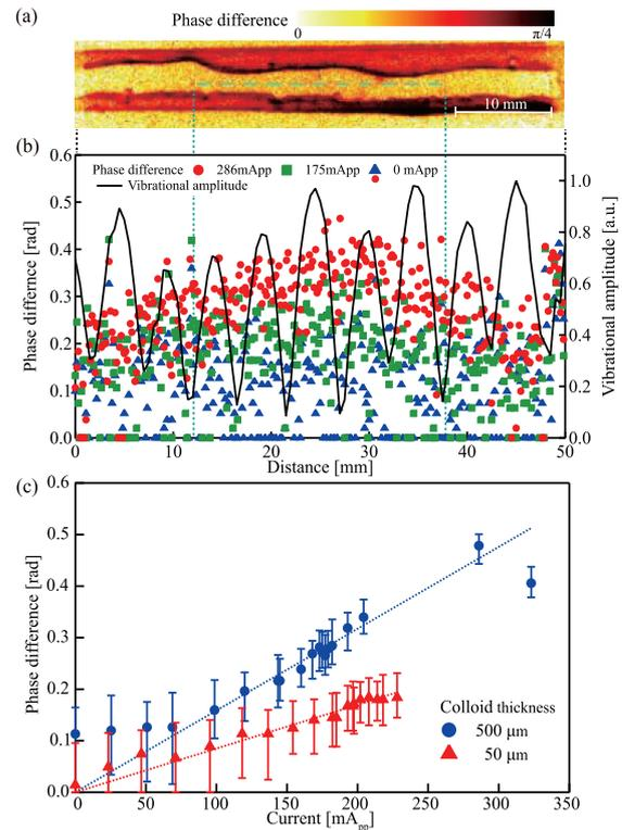
Fig.4 (a) Spatial distribution of the birefringence of the 500- $\mu$ m-thick colloid cell at 175 mA<sub>pp</sub>. (b) Distributions of birefringence and vibrational amplitude and (c) relationships between birefringence and input current at 56 kHz.
