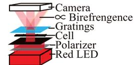
Fig. 2 Schematic of a birefringence profile.
