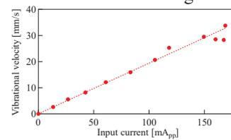
Fig. 3 Relationship between input current and vibrational velocity at 56 kHz.
